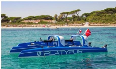
Pivoting arms connect the two hulls to the platform. Users can cruise around on the surface of the water or it can become a submersible with air supplied from an in-built compressor.
