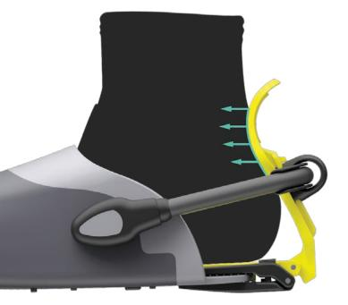
Thanks to the particular design of the heelpiece, the force exerted by the elastic is no longer concentrated in one point but distributed all the way along the back of your heel, resulting in never before experienced comfort and avoiding the annoying consequences of constant rubbing during swimming.
