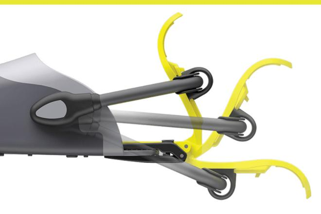
When putting on your fins, all you have to do is pull the heelpiece down until the elastic is below the fulcrum point. This way the heelpiece will remain down when you slide your foot into the fin. Finclip will then close when you gently push down with your heel.
